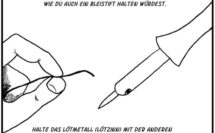
HALTE DAS LÖTMETALL (LÖTZINN) MIT DER ANDEREN HAND.
